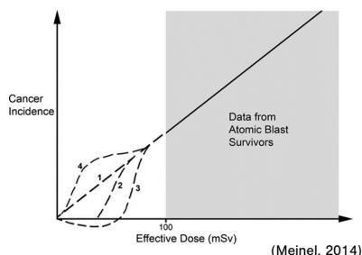
These are different models of the dose and risk relationship. Line 1 represents the linear no threshold model which is used in the UK.
