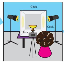
The objects are photographed in the Cubelite. External lights shine through the cube reducing shadowing. The cube also reduces reflection.
