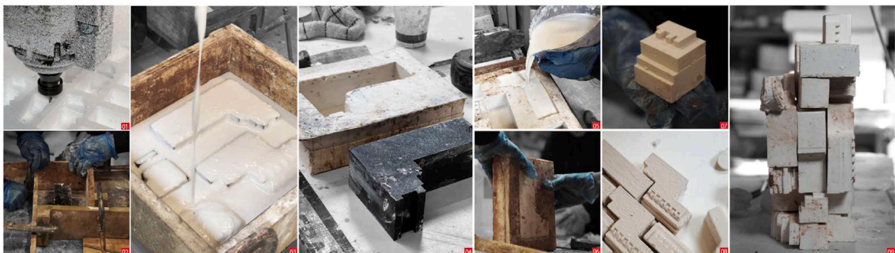
Fig. 14. Fabrication process. (1) CNC cutting is employed to produce the required geometry for mould preparation. (2–4) Alginate is used as an alternative moulding material to accelerate production. (5) A Vaseline layer is applied to prevent adhesion before plaster is poured into the alginate mould. (6) After setting, the plaster prototype is removed. (7–8) Alginate moulds yield prototypes with greater precision and surface quality compared to polystyrene forms. (9) The components are then prepared for assembly (Supplementary Video 01).
