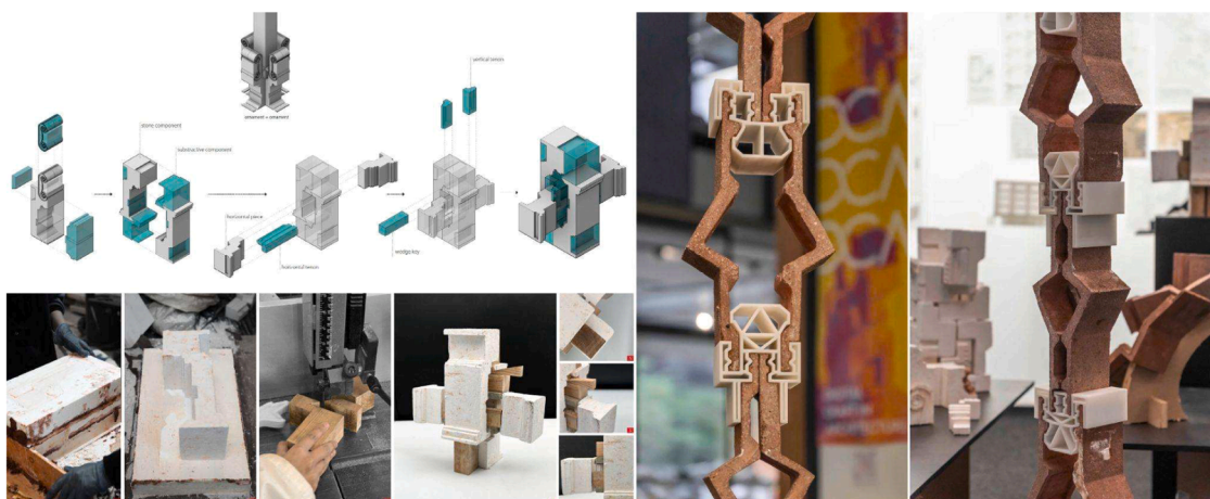
Fig. 22. Interlocking column structure using 3D printing, casting, and craft techniques. (Supplementary Material - Portfolio 01–02).
