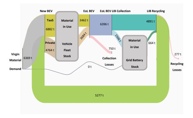
Figure 4.1: Simplified Sankey diagram for the mass flow of battery material though passenger vehicle fleet and electricity grid storage. The diagram presents the flow of lithium in tonnes for year 2035 of the 'TaaS' scenario.
