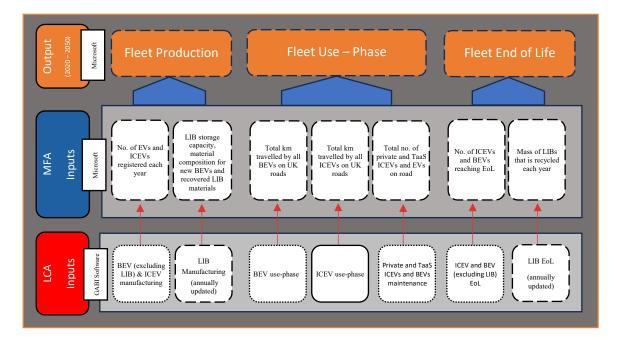
Figure 3.6: Shows the model integration framework for the fleet level environmental assessment. Solid line represents fixed inputs, dash lines represent inputs that vary for each year up to 2050 and dotted line presents inputs varying due to the evolving UK electricity grid mix only for each year up to 2050.
