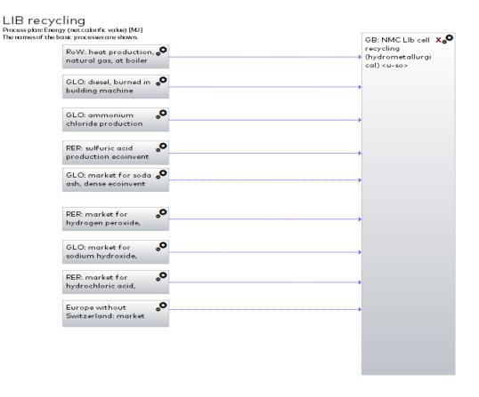
Figure F.4: Material inventory diagram for the operation of lithium battery cell recycling.
