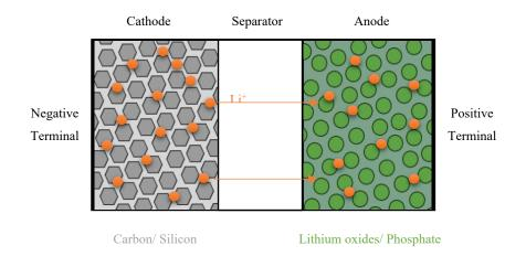
Figure 2.3: Shows the schematic of lithium-ion battery during discharge.
