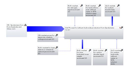
Figure F.1: Material Inventory diagram for refinement of concentrated spodumene rock in China
