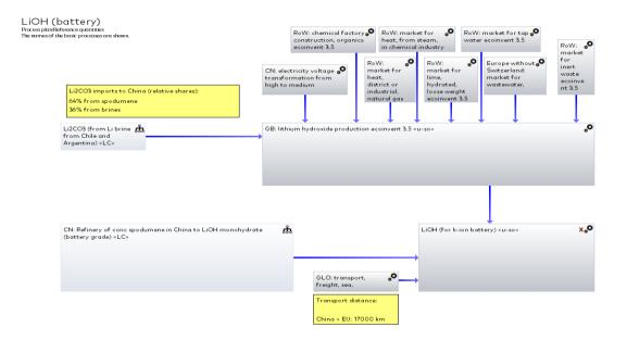
Figure F.2: Material Inventory diagram for the production of lithium hydroxide (LiOH)
