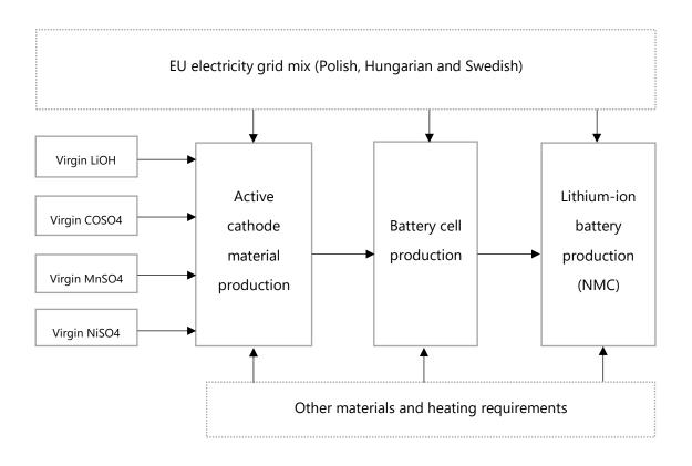
Figure 6.4: Represents the flow diagram of LIB manufacturing process in the EU. The solid lines represent the elements of manufacturing process that vary for each year due to change in required virgin materials and improvement in battery technology, whereas the dotted lines represent the static process.
