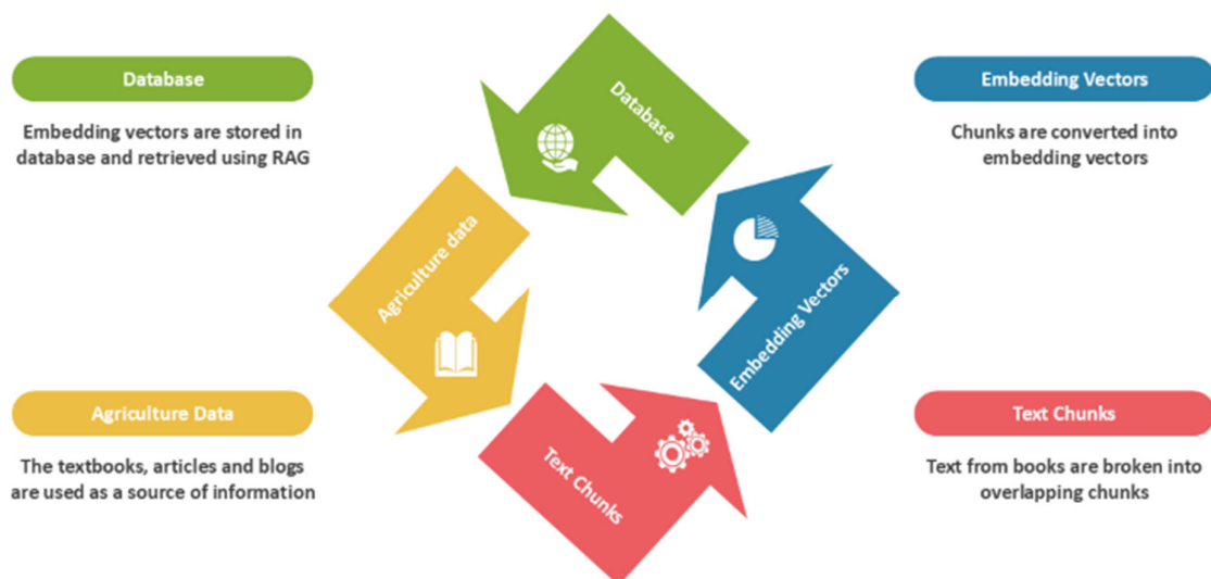
Figure 1. The workflow illustrating the transformation of agricultural textual data into embedding vectors used by AgroLLM for knowledge retrieval and response generation.
