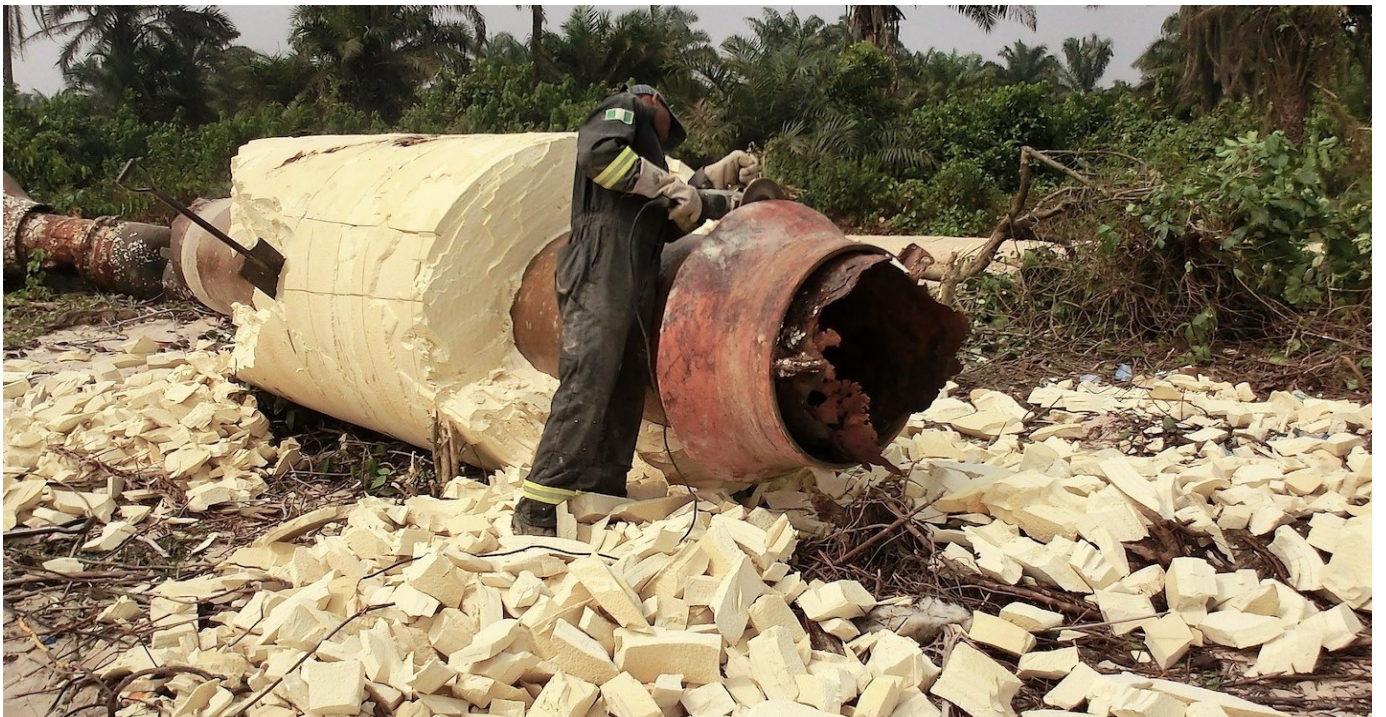
Figure 21 Wilfred Ukpong salvaging polystyrene, fiberglass and steel from a giant floater, Niger Delta, 2015
