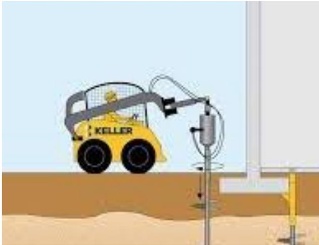
They are a ground anchoring system used as deep foundations, they are drilled into the ground with hydraulic machines and disperse the weight of a structure, and have become popular in the last decade, but being first used in the 19th Century.
