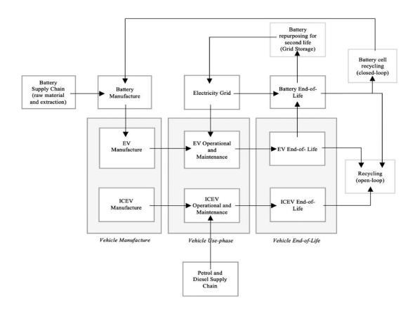
Figure 3.5: Structure of the prospective hybrid LCA model, with identification of the individual sub-models used for each of the key processes comprising the analysed system.
