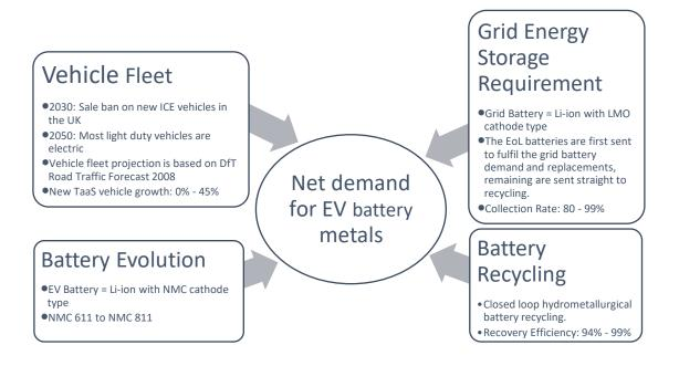
Figure 3.4: Represents the components of MFA, impacting the net demand for BEV batteries and their elements.
