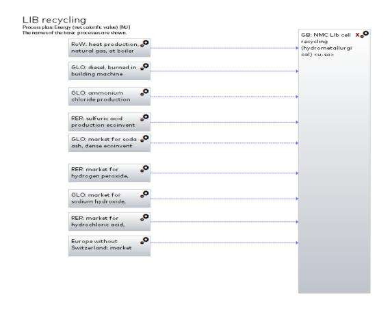
Figure F.4: Material inventory diagram for the operation of lithium battery cell recycling.
