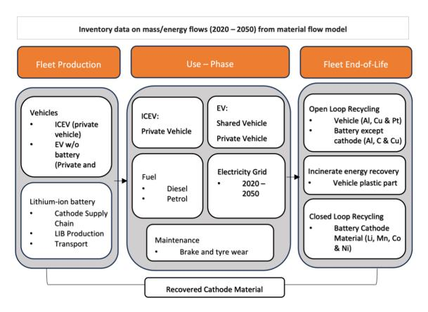
Figure 6.2: Structure of the prospective LCA passenger fleet model, with identification of the individual sub-models used for each of the key processes comprising the analysed system.
