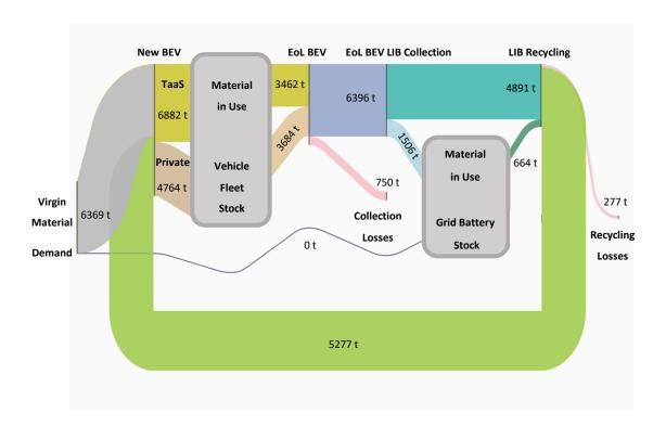
Figure 4.1: Simplified Sankey diagram for the mass flow of battery material though passenger vehicle fleet and electricity grid storage. The diagram presents the flow of lithium in tonnes for year 2035 of the 'TaaS' scenario.
