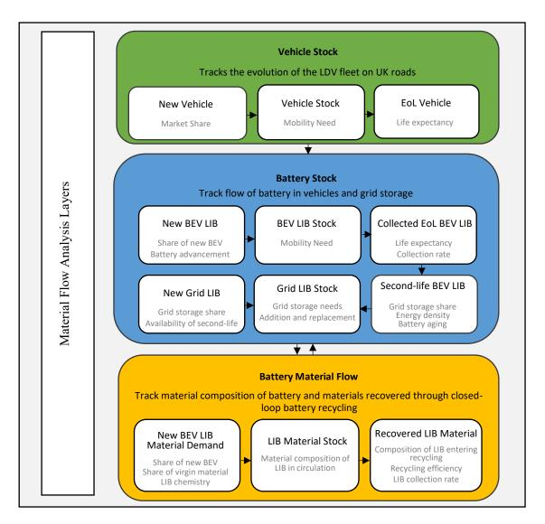
Figure 3.5 Shows the main system blocks captured by the material flow analysis.
