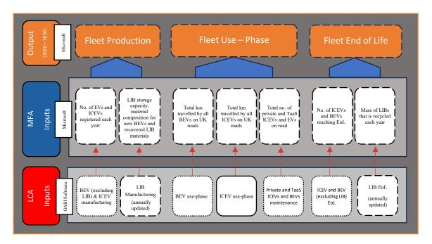
Figure 3.6: Shows the model integration framework for the fleet level environmental assessment. Solid line represents fixed inputs, dash lines represent inputs that vary for each year up to 2050 and dotted line presents inputs varying due to the evolving UK electricity grid mix only for each year up to 2050.
